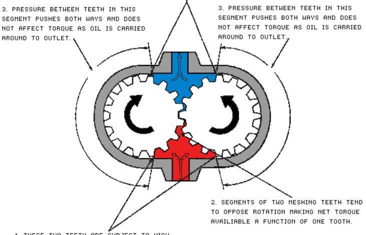
1. THESE TWO TEETH ARE SUBJECT TO HIGH PRESSURE AND TEND TO ROTATE GEARS IN DIRECTION OF ARROWS.
