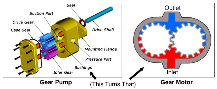
Pumps get turned by engines, motors get turned by pump displacement.
