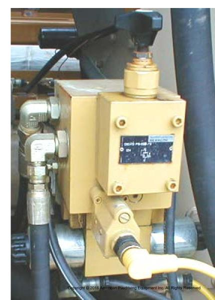
Clamp Manifold Clamp relief valve Pressure switch
