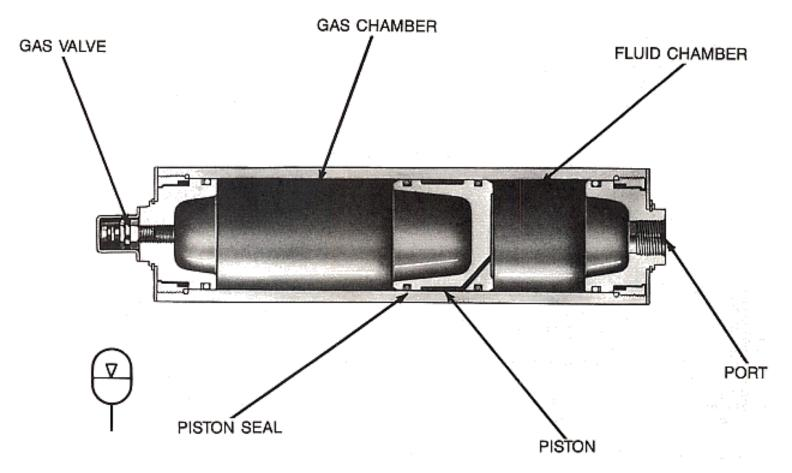
Figure 18-3. Piston accumulator is gas-charged.
