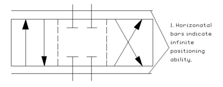
Directional valve (infinite positioning)
