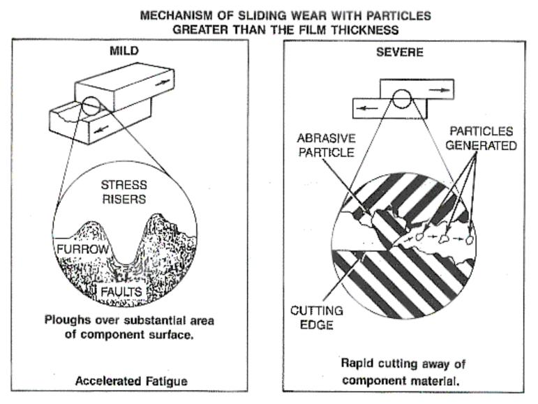
Mechanism of sliding wear with particles greater than the film thickness.
