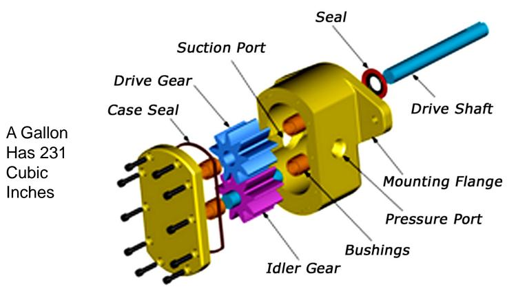
Gear sets are sized in accordance to their cubic inch of output (displacement) per revolution. Therefore, these gears could be size 3.6 which would mean 3.6 cubic inches of displacement per revolution. Total output is measured by calculating total cubic inches per minute so you would multiply 3.6 times the rotational speed per minute to get the total output.
