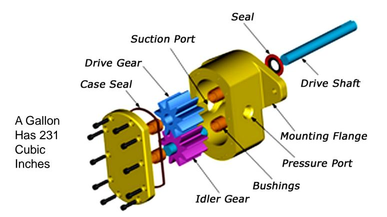
The above pump is very simple. Rotating the drive shaft causes the gears to rotate and move oil. The faster the shaft rotates, the more oil it displaces. Output is measured by counting the amount of oil it pumps in one revolution. Gears come in different widths so a wider gear set will move or pump more oil per revolution. Pump output is measured in cubic inches.
