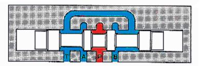
PRESSURED CLOSED-- "A" & "B" OPEN TO TANK
