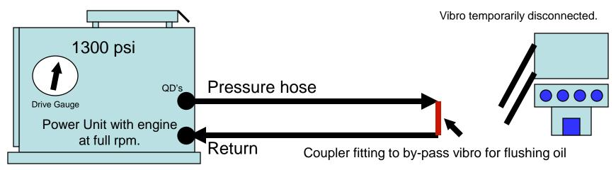
During new production of vibros and drills, we always flush the hose bundle by putting a coupler at the end of the hose bundle. This allows the oil to pass through the drive line hose an go back to the power unit through the return line. We put a in-line filter on the return line to catch the dirt.
