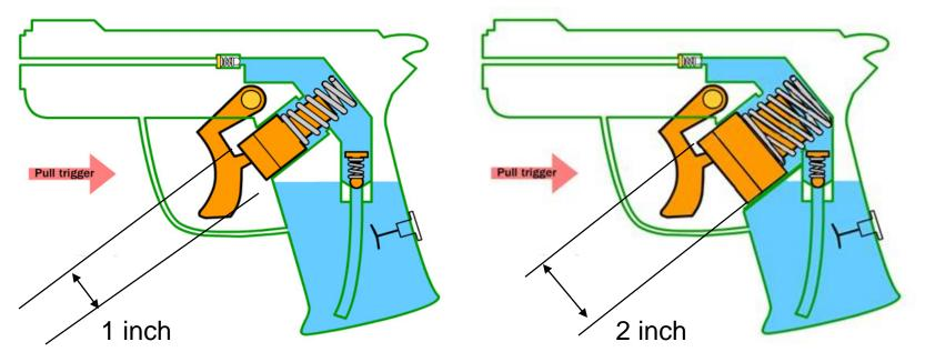
Changing piston diameter will increase volume of area. In this case, more water will be trapped in the cylinder on the gun to the right so it will spray more water per stroke. However, it will take more finger muscle to squeeze the one on the right, just as it takes more horsepower to increase pump output. Gear pumps increase with gear size, piston pumps increase with piston size or length of stroke or by adding more pistons.
