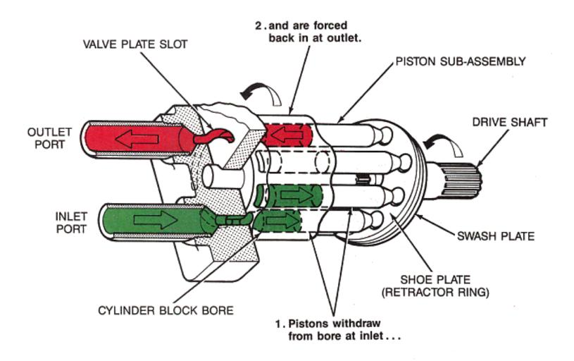
Figure 17-24. Swash plate causes pistons to reciprocate.
