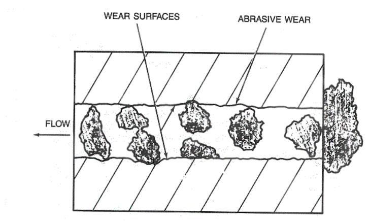
Particles, same size or slightly smaller than the clearance between moving surfaces, will interact with both surfaces to cause wear. Very large particles (right) do not normally get into critical clearance areas and thus cause little or no wear. Very small particles (less than one micrometer) usually flow through without abrading either surface.
