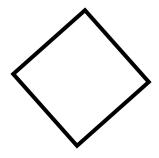
diamond – Condition apparatus (filter, separator, lubricator, heat exchanger
