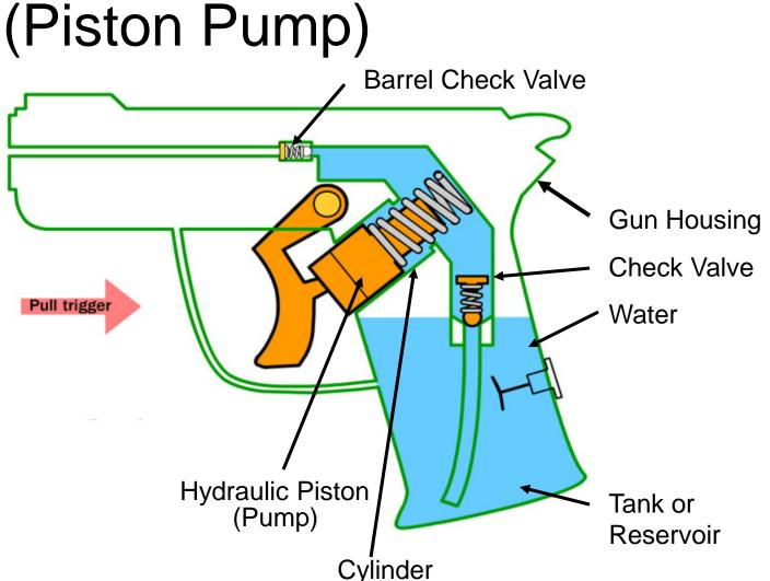
This is a simple check valve type hydraulic system just like our fuel pump on the diesel hammers; check valves that stop one direction and open in another. The injector on the diesel is really a check valve that works just like the check valve in the barrer of this squirt gun.
