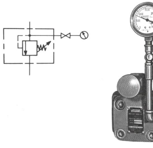
Figure 18-11. Gauge installed with shutoff valve and snubber.
