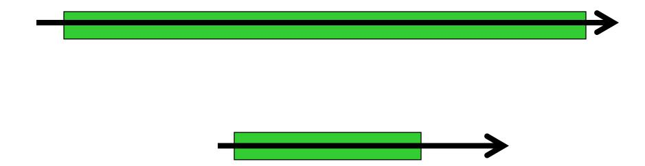
The longer the hose bundle, the more pressure drop you will have. This is why we do not want to run our vibros or drills or hydraulic impact hammers with more than 150 feet of hose. You can have so much hose that there is no available pressure left to do the work of turning the eccentrics or drill. Vibros and drills work better with larger hoses or shorter lengths.
