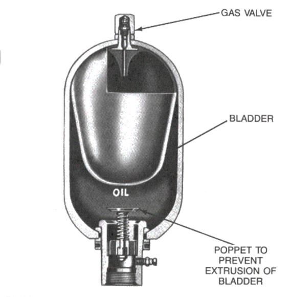
Bladder-type accumulator uses rubber separator between gas and liquid.
