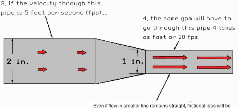
Even if flow in smaller line remains straight, frictional loss will b 16 times more than it is in the larger line.
