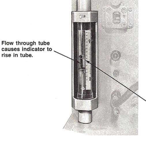
Flow rate in gpm is read directly on scale at this edge of indicator.
