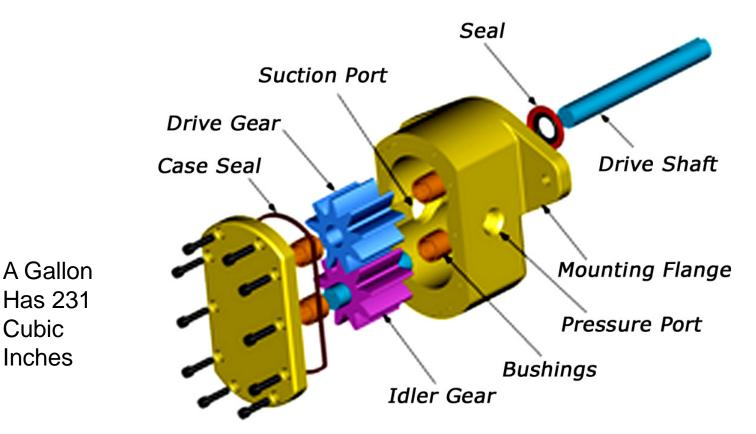
If the gears In this pump are size 3.6 then it displaces 3.6 cubic inches of oil per revolution. To find total gallons per minute (GPM) just multiply the cubic inches of displacement of the gears by the total speed the shaft turns in one minute. Example: Lets say the shaft turns 2100 rpm. The math would look like this:  $3.6 \times 2100 = 7,560$  cubic inches.
