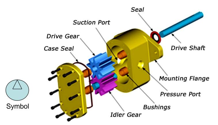
What does "fixed pump" mean? It means the pump displaces a fixed amount of oil per revolution. Much like a squirt gun. Squeeze the trigger and it pumps the same amount every time. This pump displaces the same amount every time it rotates. It pumps the moment the shaft turns and keeps pumping until the shaft stops. The faster you turn it, the more oil it displaces. You can slow down the output by slowing down the shaft speed. (turning down the rpm of the engine)
