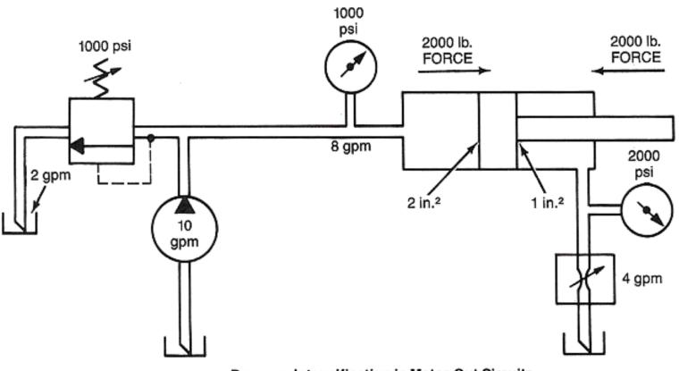
**Pressure Intensification in Meter-Out Circuits**
