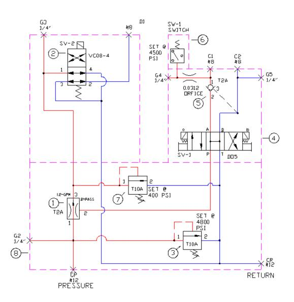
Item #5 is a pilot check valve used to trap hydraulic pressure on the closed side of the vibro clamp. There is also another one located right on the vibro clamp as well. If item #4 is in the center position, pump flow back to tank, then item #5 will trap any hydraulic pressure in the clamp close line to assure clamp remains closed.
