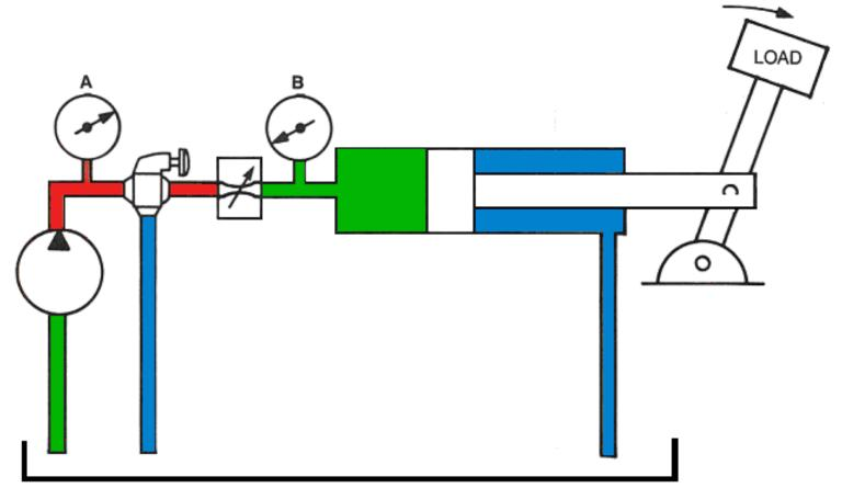
Meter-In Circuits Do Not Control Runaway Loads
