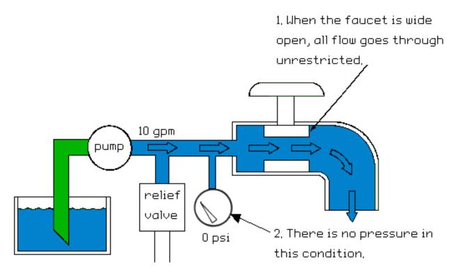
This is like our drive manifold when the vibro is not running. The oil goes through the valve and dumps right back to the tank without building any pressure mention. All Rights Reserved
