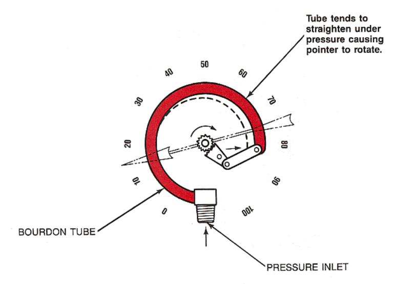
Figure 18-8. The Bourdon Tube gauge.
