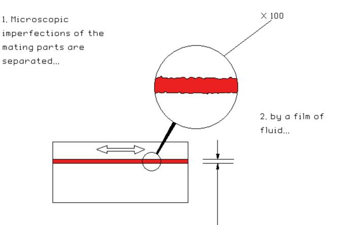
3, where clearance betwen the parts is caused by dynamic forces and fluid viscosity.
