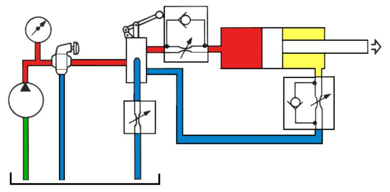
Colors based on piston extending and flow rate controlled by the rod-end valve
