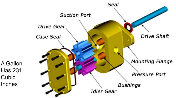
If the gears In this pump are 4.5 cubic inch then it pumps 4.5 cubic inches per revolution. To find total gallons per minute (GPM) just multiply the cubic inches of the gears by the total speed the shaft turns in one minute. Example: Lets say the shaft turns 2100 rpm. The math would look like this:  $4.5 \times 2100 = 9450$  cubic inches.
