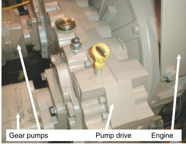
Do not always assume that the pump drive is turning at the same rpm as the engine. Ratios are stamped on the pump drive.
